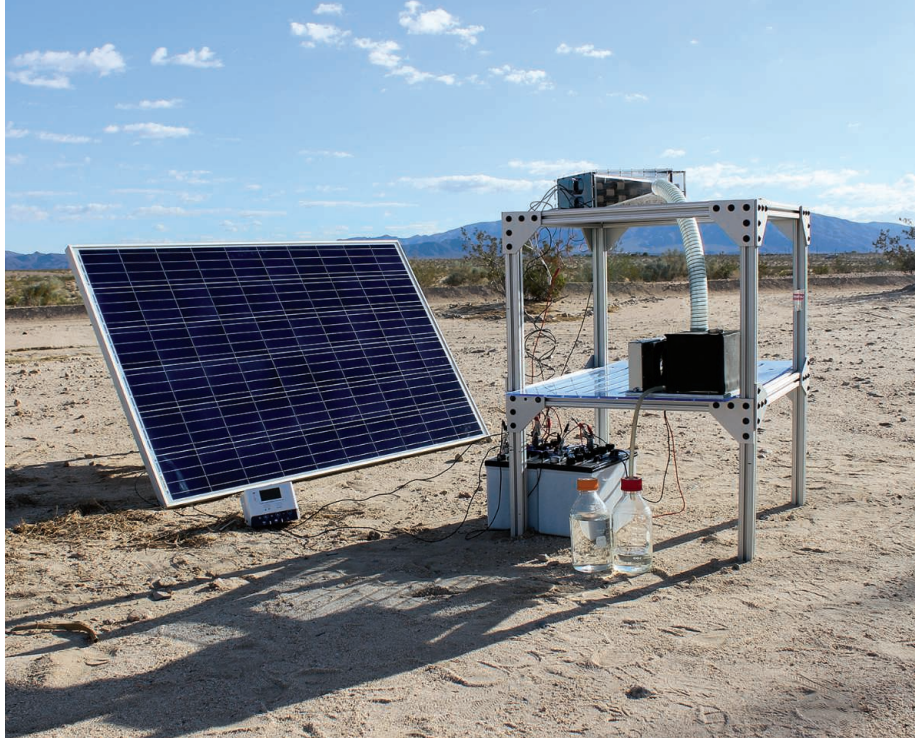
A solar panel powers a device that harvests water from the air in California's Mojave Desert.
