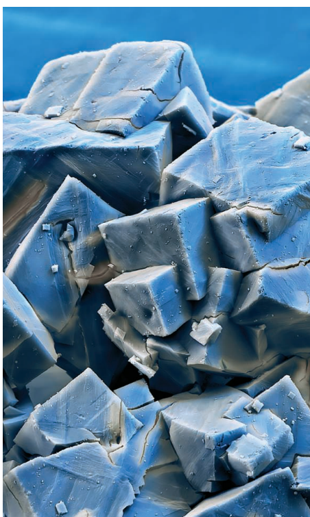
Crystalline metal-organic framework (MOF) materials under development at BASF. The company is working to scale up the production of MOFs to store natural gas.
