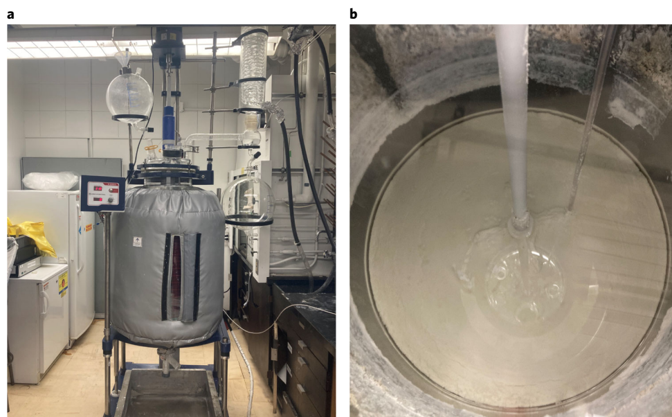
Fig. 4 | A 3-kg-scale synthesis of MOF-303 in a 200 L reaction vessel. a , Reaction setup of the vessel equipped with an addition funnel, a condenser and an overhead rotor connected with a spinner. b , Formation of a white precipitate after refluxing for 6 h.
