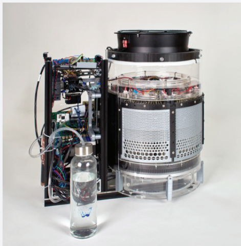
Figure 3. MOF Water Harvester. A working prototype for water harvesting from air based on 100 g of MOF. It is capable of producing 4 L per day with minimum energy input. The MOF is based on aluminum and can remain in the device for the lifetime of the electronics (6 years). Image: courtesy of Water Harvesting Inc.
