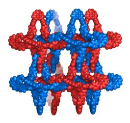
The team achieved postsynthetic removal of the copper(I) ions (up to 90 %) by adding aqueous KCN to obtain the corresponding COF. The researchers anticipate that such interlocking structures could be useful in flexible materials that retain their robustness and resilience. This could have applications, e.g., in soft robotics, bullet-proof structures, or materials that require stiffening on demand.
